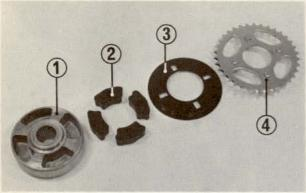
Fig. 27 (1) Damper case (2) Sprocket damper
