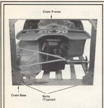
STEP 5—Remove four bolts (two on each end) attaching steel crate frame to crate base and carefully lift off frame.
