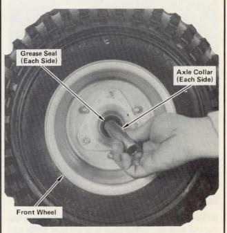
STEP 21—Insert an axle collar into front wheel grease seal on each side. Inflate front tire to 2.2 psi.
