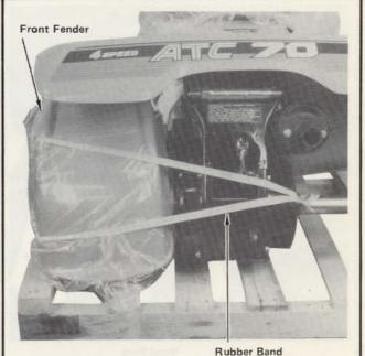
**STEP 8**—Remove front fender from under rear fender by removing rubber band.
